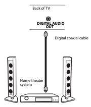
3 Connect the other end of the audio cable to the digital coaxial input jack on the home theater system.
